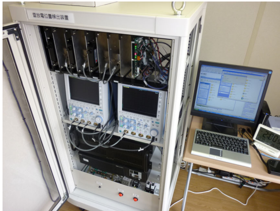
Fig. 4. Lightning observation system.
