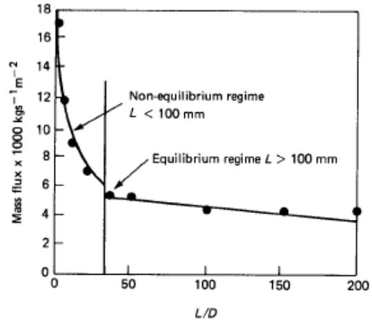
Figure 6: Empirical equation fit with experimental Freon-11 data
