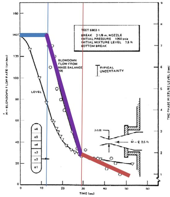
Figure B-II: Blowdown response for large blowdown vessel test 5803-1
