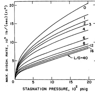
Fig. 8. Maximum discharge rates of saturated water for 0.25-in. I.D. tube.
