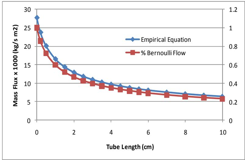
Figure 5: Theoretical saturated chlorine flow rate when the tube length is between 0 – 10 cm
