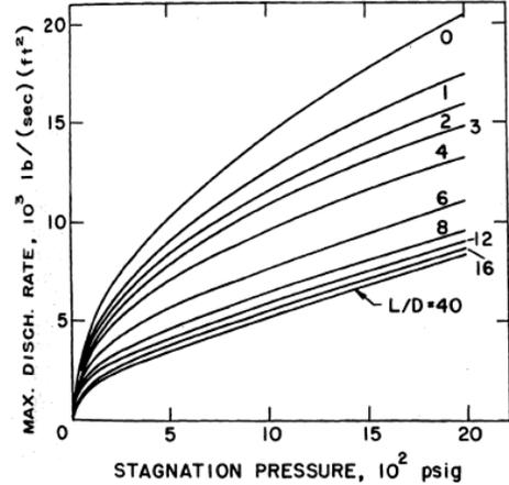
Figure 4: Graphs from the article showing that small tube lengths impact mass flow rate
