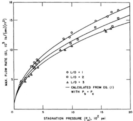
Fig. 4. Maximum discharge rates of saturated water for 0.25-in. I.D. tube.
