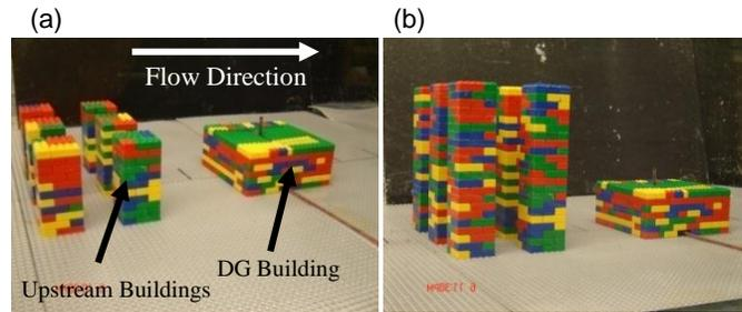
**Fig.3 (a) DG and single storey upstream buildings modeled in water channel using Lego. (b) DG and double storey upstream buildings modeled in water channel using Lego**
