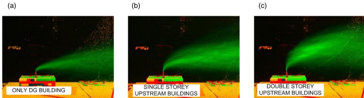
**Fig. 6 Plume visualizations for (a) Only DG building (No upstream buildings) (b) Single storey upstream buildings (c) Double storey upstream buildings**
