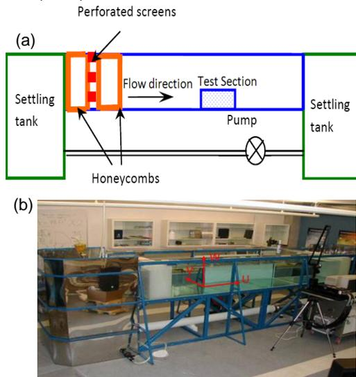
**Fig. 1 (a) Water Channel Schematic (b) Water Channel facility at University of California, Riverside**
