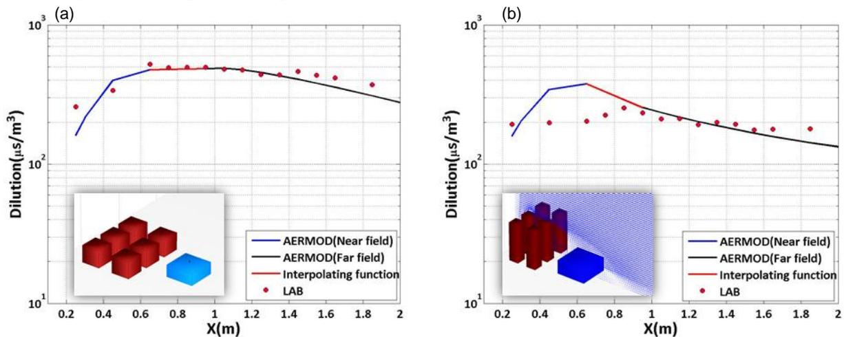
Fig.8 Modified AERMOD vs. Observations for (a) Single Storey Upstream Buildings (b) Double Storey Upstream Buildings (Red dots(●) represents the observed ground level concentrations, solid blue line(—) represents near field AERMOD predictions, solid black line(—) represents far field AERMOD predictions and solid red line(—) represents interpolating function predictions on ground level concentrations)
