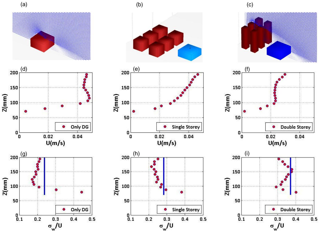
**Fig. 5 Schematic of laboratory setting for (a) Only DG building case (b) DG and single storey upstream building case (c) DG and double storey upstream building case , Velocity profile close to stack for (d) Only DG building case (e) DG and single storey upstream building case (f) DG and double storey upstream building case , Vertical turbulent intensity for (g) Only DG building case (h) DG and single storey upstream building case (i) DG and double storey upstream building case**
