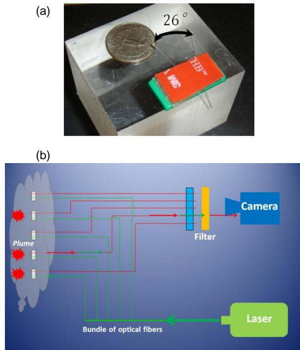
**Fig. 2 (a) Optical Fiber Sensor (b) Schematics of the concentration measurement system (green fibers are emitting fibers and red fibers are receiving fibers)**
