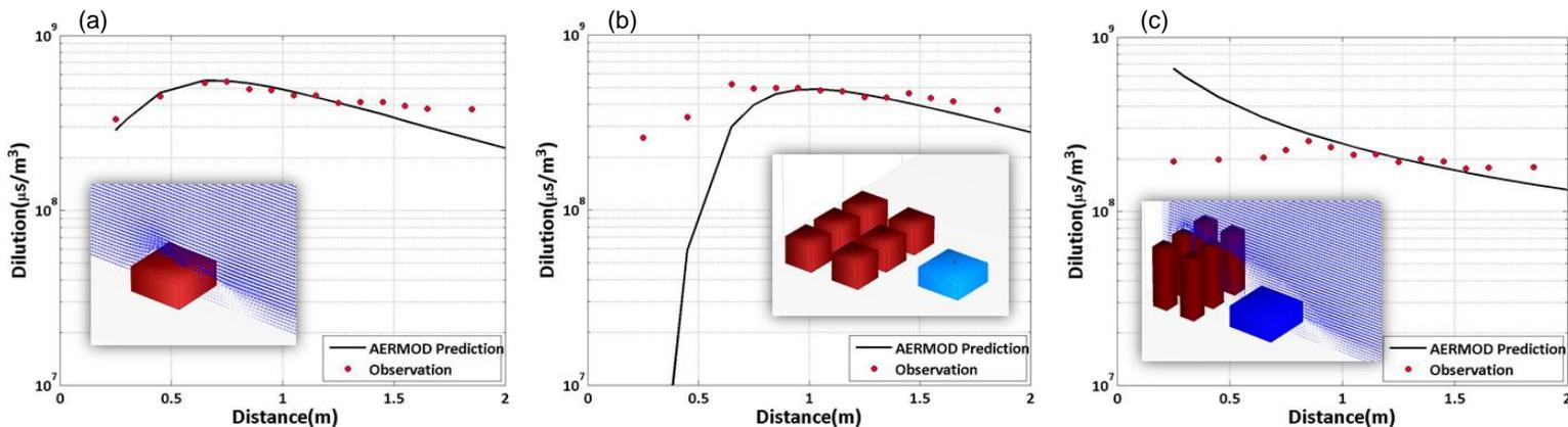
**Fig. 4 Effect of the presence of the upstream building on the ground level dilution and prediction by AERMOD (a) No upstream buildings (b) Single storey upstream buildings (c) Double storey upstream buildings (Red dots(●) represents the observed ground level concentrations and solid black line(—) represents AERMOD predictions on ground level concentrations)**
