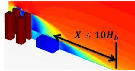
Fig.7 Schematic of the near field region in the modified version of AERMOD dispersion model
