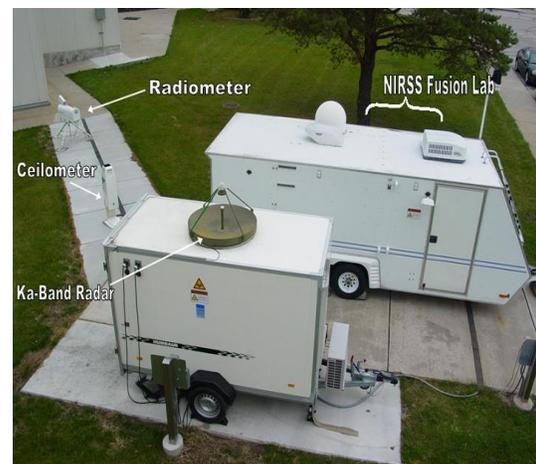
**Figure 2.** Image of the NIRSS hardware located at the NASA Glenn Research Center in Cleveland, Ohio.
