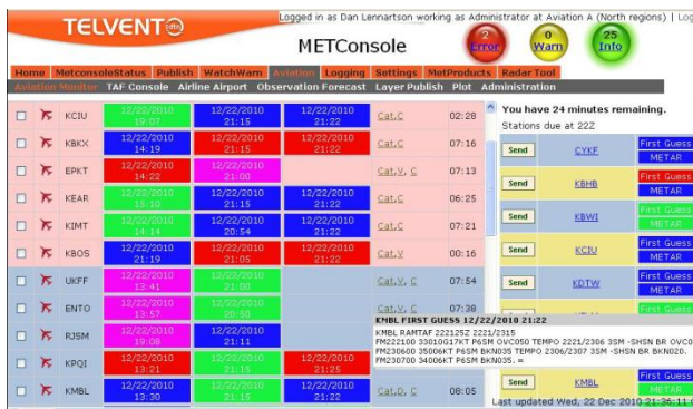
Figure 2: The IRM is activated on a schedule where a forecaster can mouse over a first guess automated initial forecast and either send it directly with the button or click the ICAO to launch TAFConsole to perform an edit and send.
