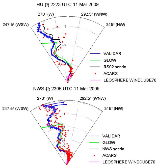
Figure 19. Wind direction of radiosonde, GLOW, VALIDAR, and ACARS during the sonde flights in the cold front case analysis time period. Range rings are height in km ASL and radials are wind directions.
