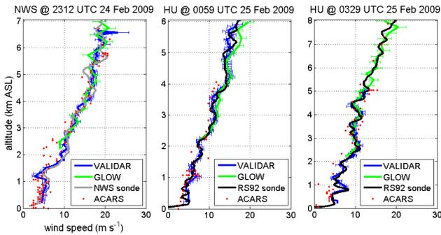
Figure 4. Wind speed of radiosonde, GLOW, VALIDAR, and ACARS during the sonde flights in the clear sky case analysis time period.
