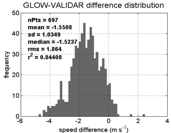
Figure 15. Cold front case GLOW-VALIDAR wind speed difference distribution.
