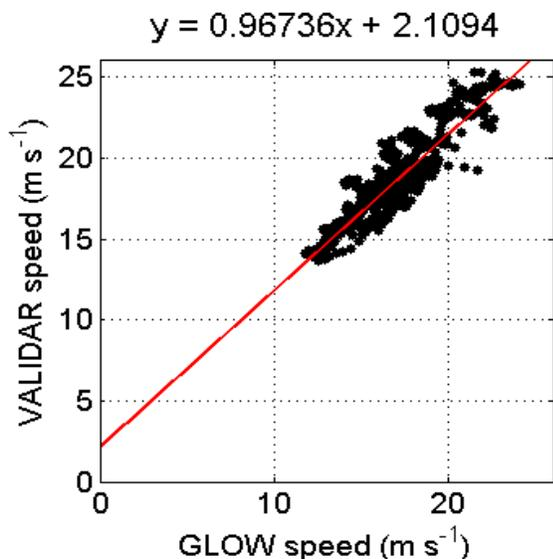
Figure 16. Linear regression of cold front GLOW-VALIDAR points.
