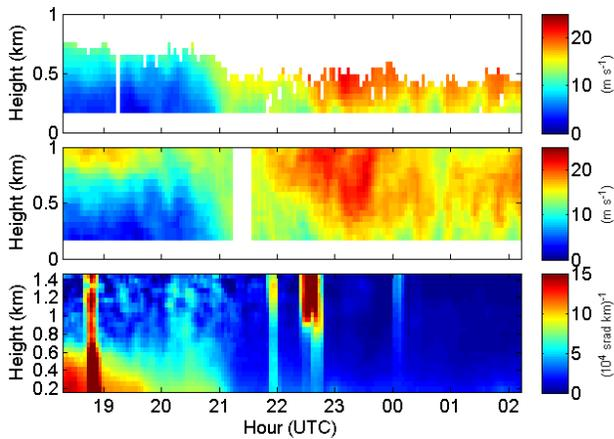
Figure 21. (top) LEOSPHERE WINDCUBE70 wind speed with 9-point horizontal moving average interpolated to VALIDAR resolution, (middle) VALIDAR wind speed with 3-point horizontal moving average and (bottom) ceilometer backscatter interpolate to VALIDAR resolution.
