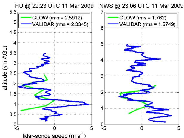
Figure 17. Difference of lidar minus radiosonde speed from profiles that are matched in time and height and interpolated to the lidar levels.
