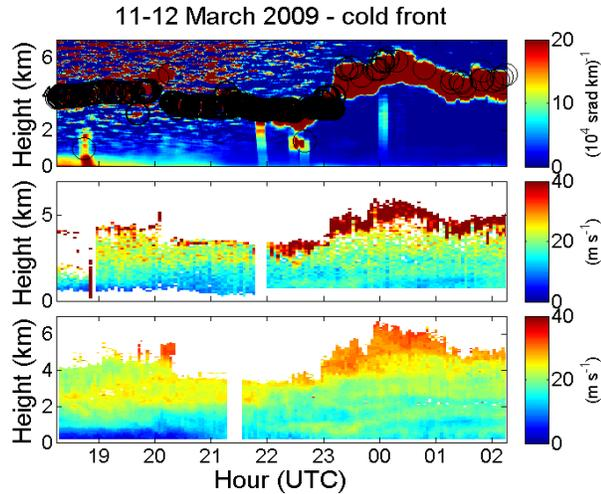
Figure 12. Wind lidar and ceilometer data for the cold front case. (top) ceilometer backscatter with ceilometer-indicated cloud base (O), (middle) GLOW 3-minute shot averaged wind speed profiles at 100 m vertical resolution, and (bottom) VALIDAR wind speed.
