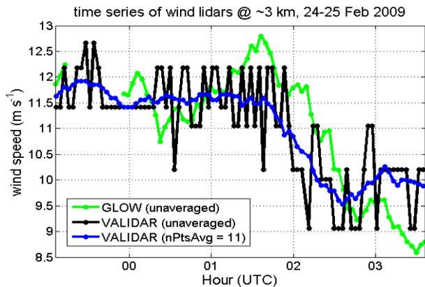
Figure 7. Time series of GLOW (33-minute shot average) and VALIDAR data at the VALIDAR height level nearest to 3 km. The GLOW data are interpolated to this height. The blue line is an 11-point moving average of the VALIDAR data.
