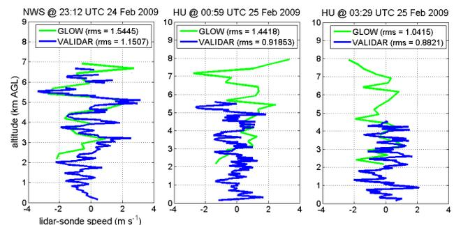
Figure 3. Difference of lidar minus radiosonde speed from profiles that are matched in time and height and interpolated to the lidar levels.
