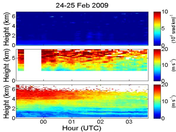
Figure 6. Wind lidar and ceilometer data for clear sky case. (top) ceilometer backscatter, (middle) GLOW 9-minute shot averaged wind speed profiles, and (bottom) VALIDAR wind speed.
