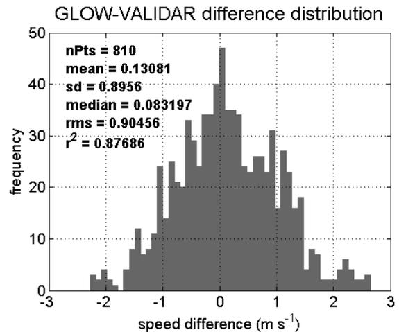
Figure 9. Clear sky case GLOW-VALIDAR wind speed difference distribution.
