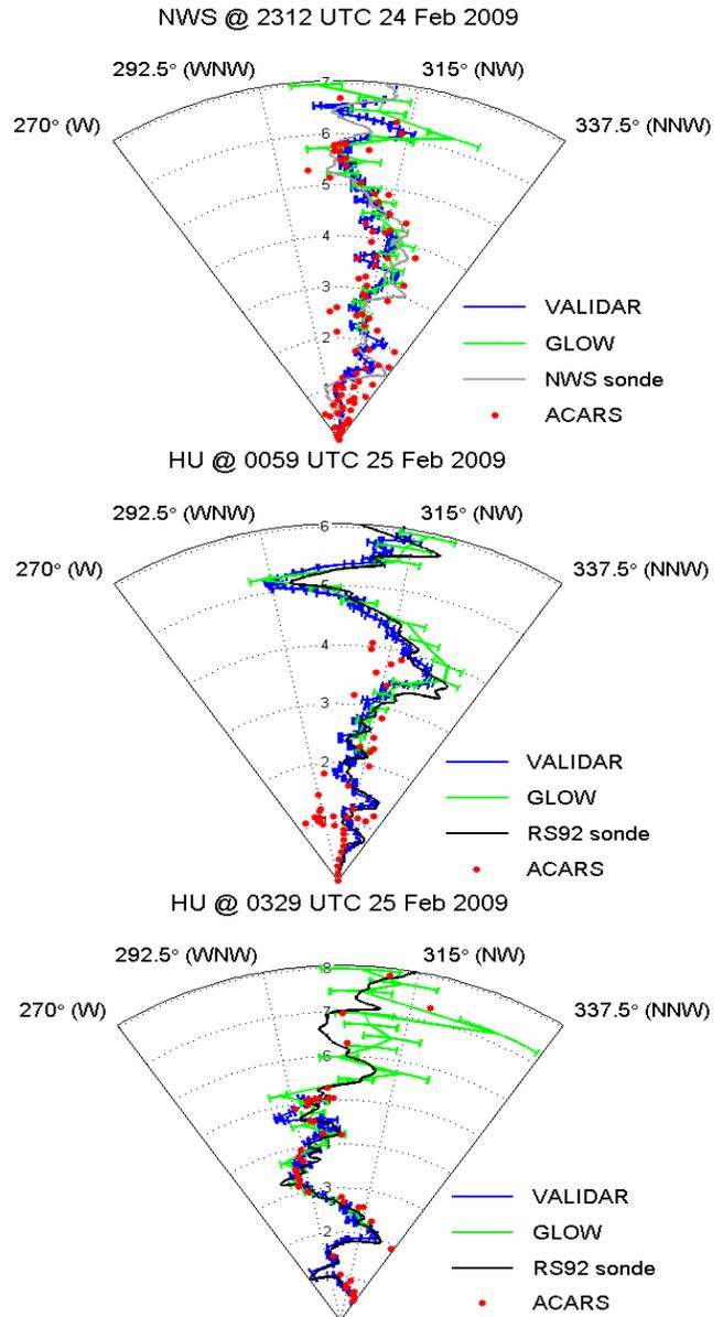
Figure 5. Wind direction of radiosonde, GLOW, VALIDAR, and ACARS during the sonde flights in the clear sky case analysis time period. Range rings are height (in km above sea level) and radials are wind direction (in degrees from true north).
