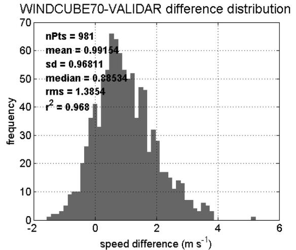
Figure 23. Cold front case WINDCUBE70-VALIDAR wind speed difference distribution.
