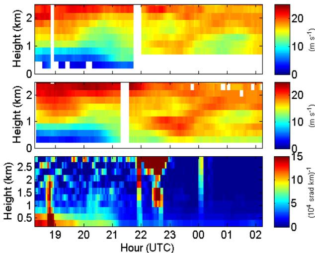
Figure 13. Time-height interpolated data for 11-12 March 2009. (top) GLOW (33-minute shot average) wind speed, (middle) VALIDAR wind speed with 11-point horizontal moving average interpolated to GLOW resolution, and (bottom) ceilometer backscatter interpolated to GLOW resolution.
