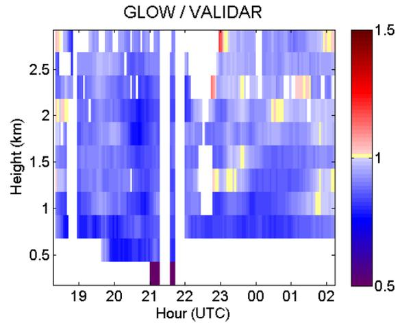
Figure 14. Ratio of GLOW to VALIDAR wind speed for the cold front case.
