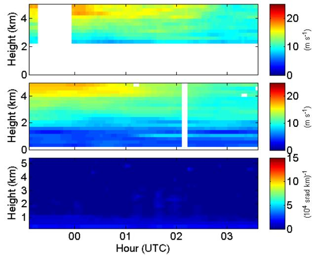
Figure 8. Time-height interpolated data for 24-25 Feb 2009. (top) GLOW (33-minute shot average) wind speed, (middle) VALIDAR wind speed with 11-point horizontal smoothing interpolated to GLOW resolution, and (bottom) ceilometer backscatter interpolated to GLOW resolution.
