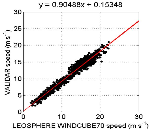
Figure 22. Linear regression of cold front WINDCUBE70-VALIDAR points.
