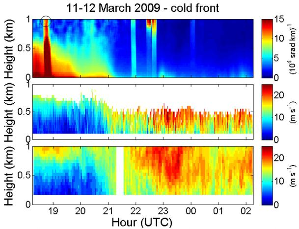
Figure 20. Wind lidar and ceilometer data for the cold front case. (top) ceilometer backscatter with ceilometer-indicated cloud base (O), (middle) LEOSPHERE WINDCUBE70 wind speed, and (bottom) VALIDAR wind speed.
