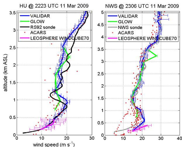
Figure 18. Wind speed of radiosonde, GLOW, VALIDAR, and ACARS during the sonde flights in the cold front case analysis time period.
