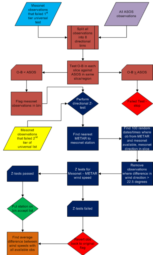
Fig. 5: Decision tree illustrating the directionally dependent accept list procedure.
