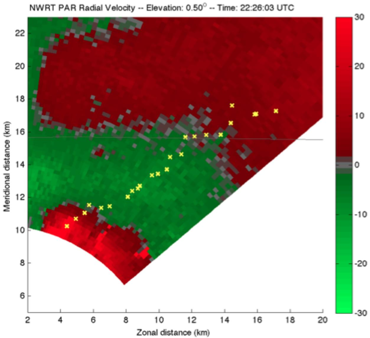
Figure 5. Same as Fig. 3, except showing the tornado path obtained using 30-s updates.
