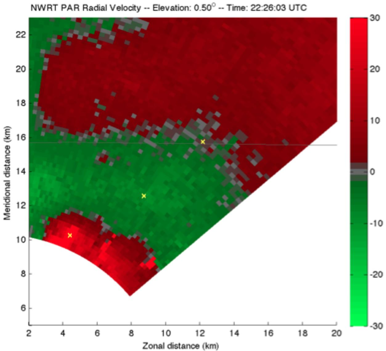
Figure 3. A circulation track obtained using NWRT PAR radial velocity from 2231–2238 UTC on 10 May 2010. The data was degraded to produce 4-min updates at the  $0.5^\circ$  elevation. Positions of the circulation center are indicated by yellow x's.
