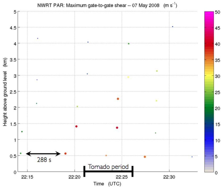
Figure 1. Time-height evolution of gate-to-gate shear during the 07 May 2008 EF-0 tornado. These points were measured using NWRT PAR data and a simulated VCP 12 scan time of approximately 4 min. Colors represent the magnitude of gate-to-gate shear measured from each elevation scan. The tornado was on the ground from 2221–2226 UTC.
