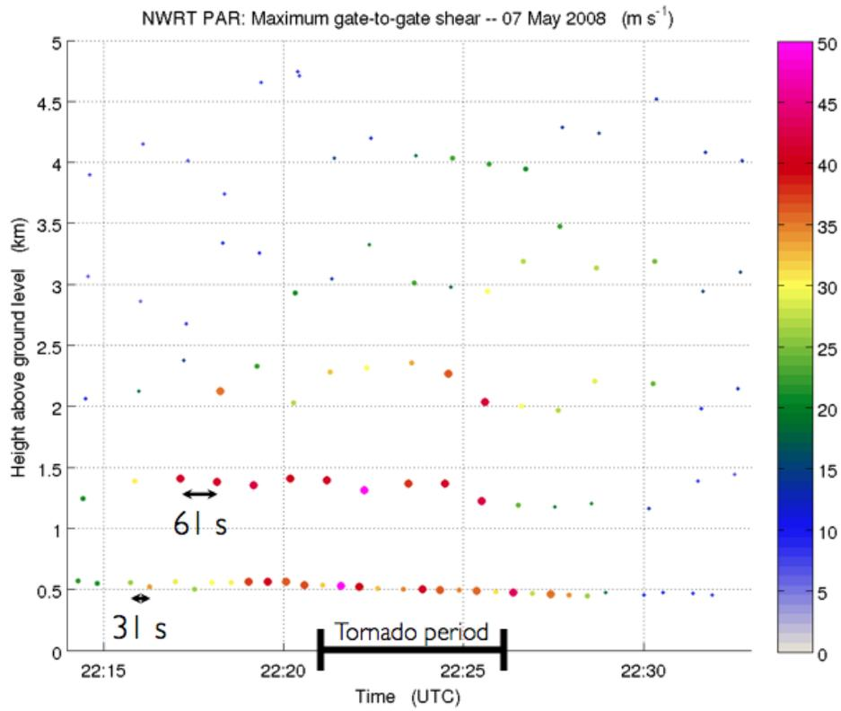
Figure 2. Same as Fig. 1, except showing native NWRT PAR resolution. The lowest elevation ( $0.5^\circ$ ) was sampled at a 30-s interval, while a complete volume was obtained in 60 s.
