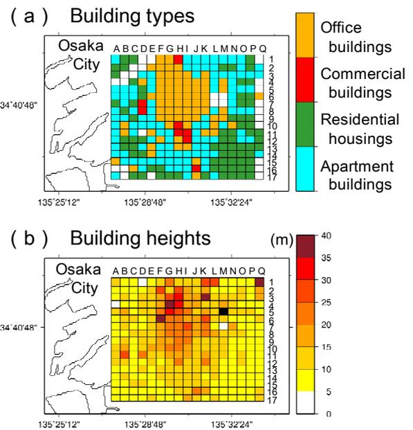
Fig. 3 Mesh maps of (a) main building types and (b) averaged building heights. A black-toned mesh in (b) indicates the maximum building height of 69.8 m of our region.
