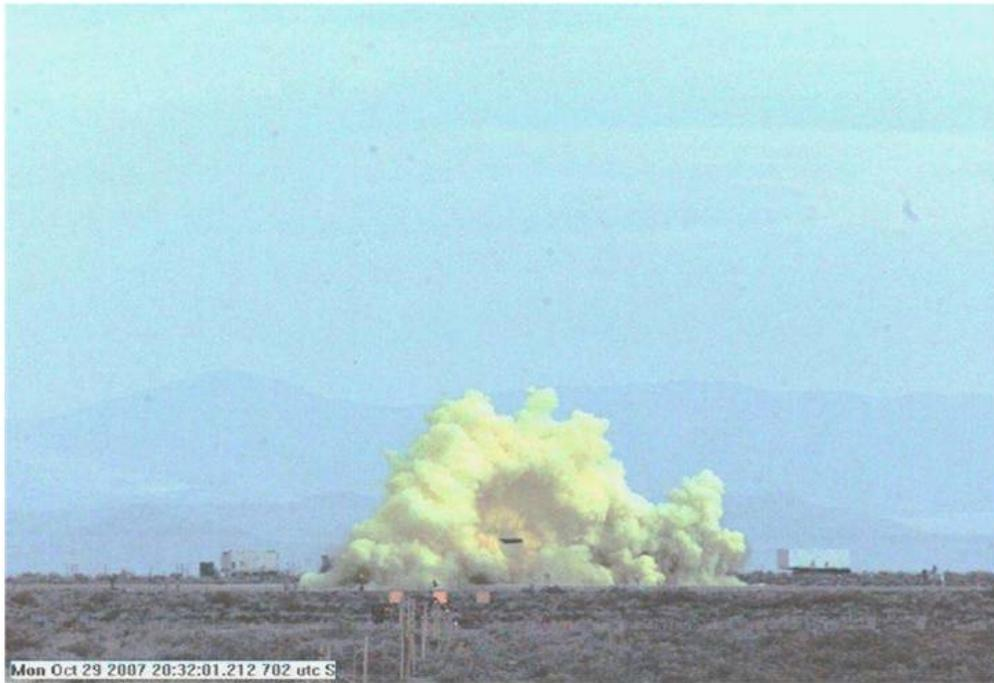
**Figure 3.** Photo of Wild Stallions chlorine cloud during the release phase with a two-phase jet, from Trial 7 with a rotating tank.
