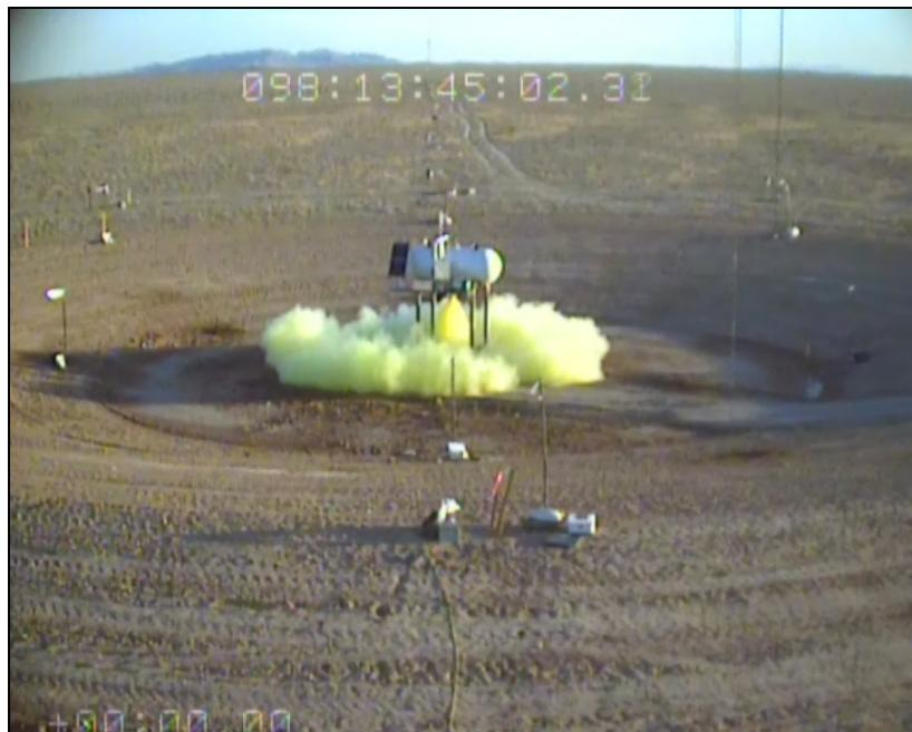
**Figure 6.** Jack Rabbit chlorine release site, showing the 50 m diameter by 2 m deep depression and the tank set-up. This is the one-ton pilot release (Trial 2, see Tables 3 and 4). The photo was taken about 2 seconds after the chlorine release began. The downward pointing two-phase momentum jet is seen, and the horizontal “wall-jet”, extending radially, is just becoming evident. Photo courtesy of Dugway Proving Ground.
