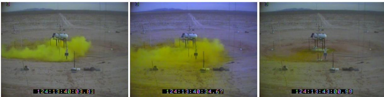
**Figure 8.** Jack Rabbit Trial 6 (see Tables 3 and 4) chlorine cloud, at 3 seconds (left), 34 seconds (center) and 180 seconds (right) after the release began. This trial had larger wind speeds (6.2 m/s vs 0.6 m/s) than Trial 2, and the cloud here is observed to not be held-up in the depression. Photos courtesy of Dugway Proving Ground.
