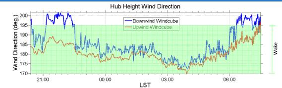
Figure 9: Upwind & downwind 80m LIDAR wind direction for July 16-17, 2011. Turbine wake exists over the downwind LIDAR for wind directions of 167° to 195° assuming a 5° wake expansion.
