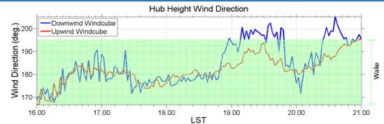
Figure 6: Upwind & downwind 80m LIDAR wind direction for July 23, 2011. Turbine wake exists over the downwind LIDAR for wind directions of 167° to 195° assuming a 5° wake expansion.
