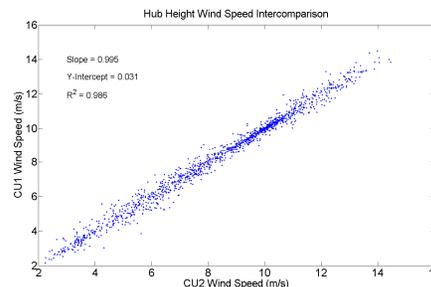
Figure 5: Horizontal wind speeds at 80m for the two Windcubes during the 2 day intercomparison period
