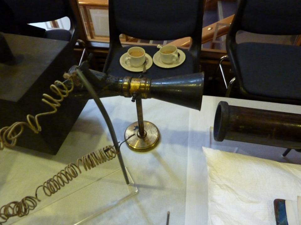
When heated, a thermopile produced a current detected by a galvanometer. T
