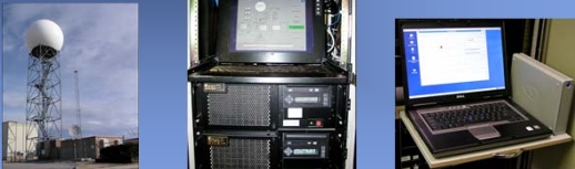
Returned Signals → ORDA → Level I Recorder
