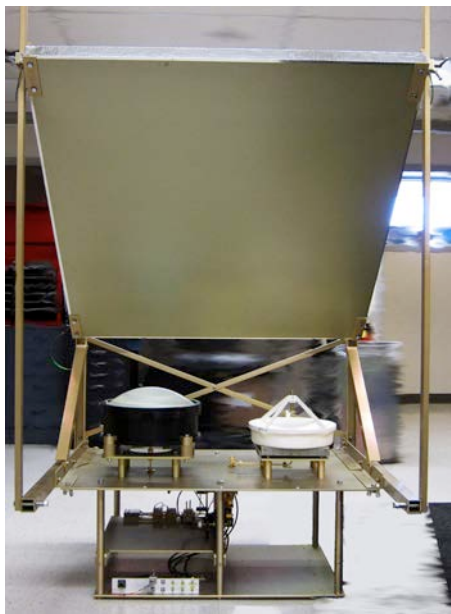
Figure 11. The transmit and receive antennas, with a horizontal reflector for ground testing.
