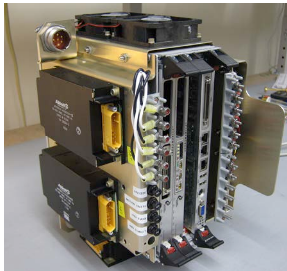
Figure 12. The host computer chassis. The FPGA transceiver is mounted in the carrier card; second slot from the left.
