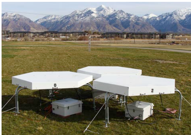
Figure 8. The spaced antenna array.
