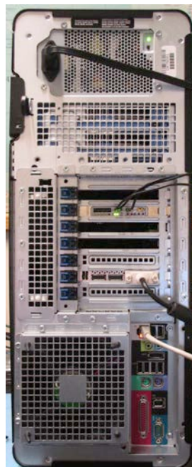
Figure 9. The host workstation. The FPGA transceiver is the card with the three attached coax cables.
