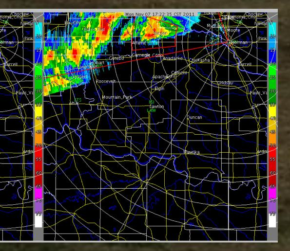
The algorithm did a good job tracking the boxed part of the squall line, repositioning the antenna when the left side of tracking box reached the left scan sector boundary.
