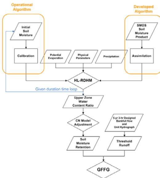
Figure 6 Flow chart of verification and comparison of operational GFFG system and satellite based developed algorithm GFFG
