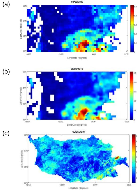
Figure 4 Arkansas red river basin area soil moisture from (a) SMOS 0.25 degree (b) SMOS interpolated to 4 km x 4 km (c) upper zone water content ratio from HL-RDHM on September 6<sup>th</sup>, 2010
