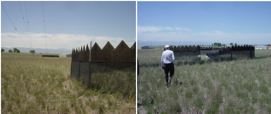
Figure 17. Eddy fences at the abandoned NOAA ISNet site at the Boulder Atmospheric Observatory (BAO) in Colorado.
