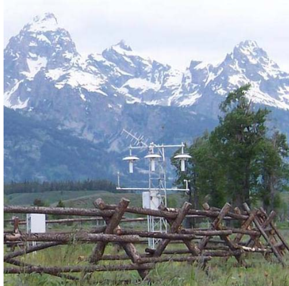
Figure 1. Three radiation shields housing and fan aspirating three independent platinum resistance thermometers at the WY Moose 1 NNE USCRN station in Grand Teton National Park.
