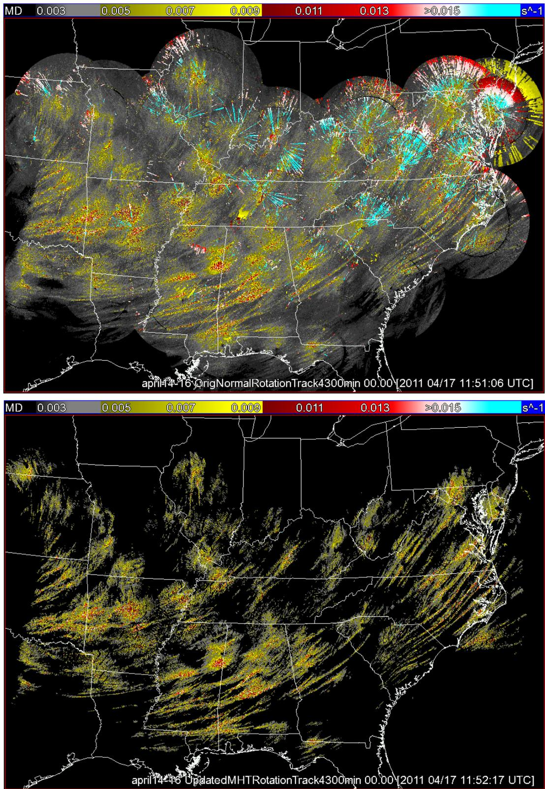
Figure 4: Top: Rotation tracks made from maximum azimuthal shear fields between 0-3km AGL from 12Z on 14 April 2011 to 12Z on 17 April 2011. Bottom: The same rotation tracks after the quality control was performed. Note the most isolated tracks and removal of the radial “spikes”.
