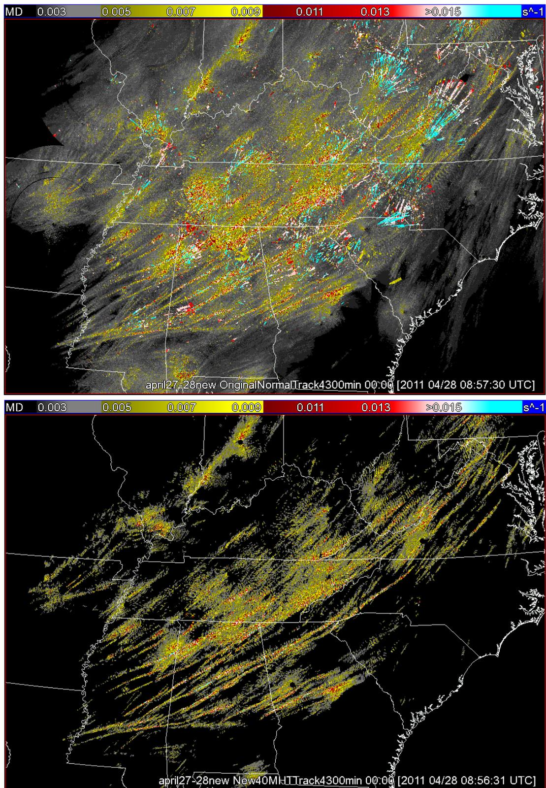
Figure 5: Top: Rotation tracks made from maximum azimuthal shear fields between 0-3km AGL from 16Z on 27 April 2011 to 08Z on 28 April 2011. Bottom: The same rotation tracks after the quality control was performed. Note the most isolated tracks and removal of the radial "spikes".
