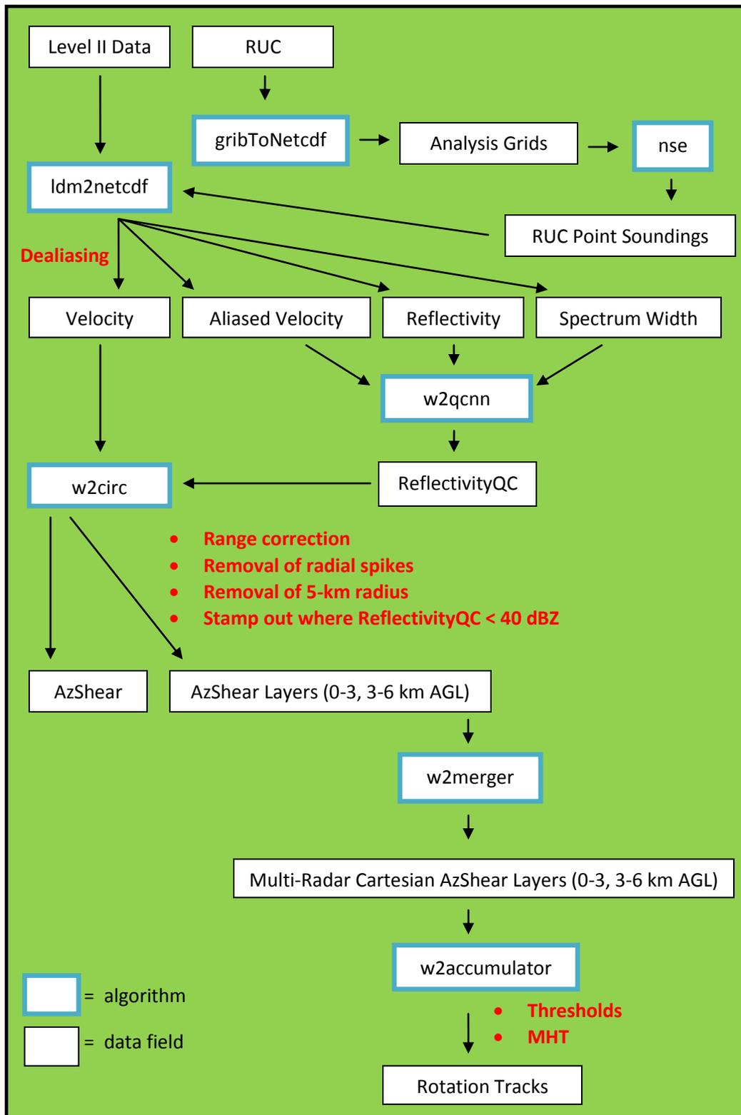
Figure 2: Data flow used to create 2D maximum azimuthal shear rotation tracks when incorporating the new dealiasing and quality control techniques. The new techniques are written in red next to the step where they are applied.
