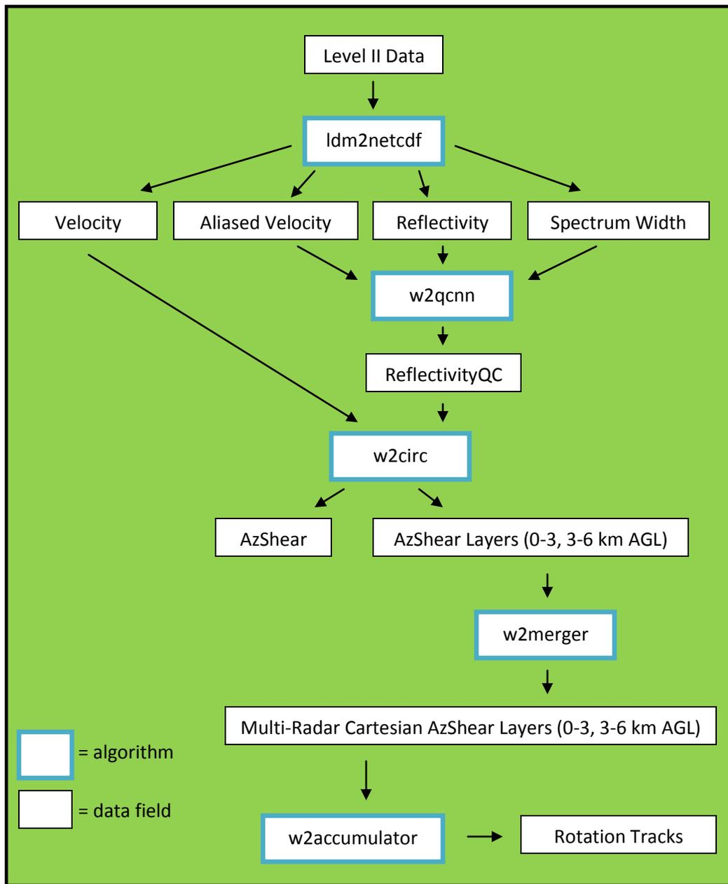
Figure 1: Data flow used to create 2D maximum azimuthal shear rotation tracks.
