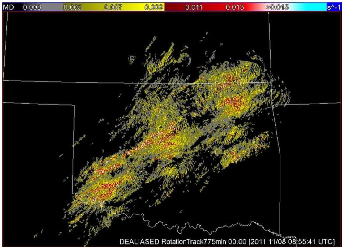
Figure 6: Top: Rotation tracks made from maximum azimuthal shear fields between 0-3km AGL from 20Z on 07 November 2011 to 09Z on 08 November 2011. Bottom: The same rotation tracks after the quality control was performed.
