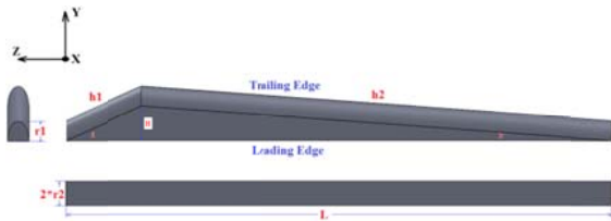
Figure 5: Geometry of a simplified blade model. A blade is composed of three basic shape objects: elliptical cylinder, rectangular plate and triangular plate.
