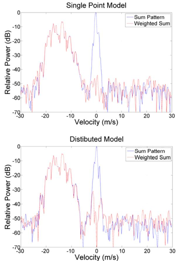
Figure 6. Spectra showing the performance of spatial filtering for both a single point and distributed clutter model using 18 sidelobe cancellers.
