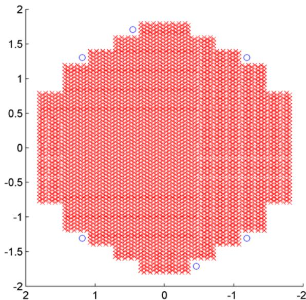
Figure 2. Locations of the main array antenna elements and sidelobe canceller receive antennas.
