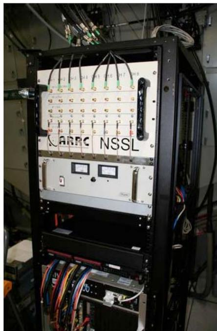
Figure 1. A picture of the multi-channel receiver instrument rack installed at the National Weather Radar Testbed.
