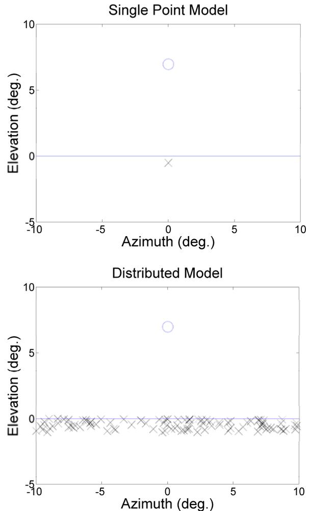
Figure 4. Comparison between the single point and distributed clutter models.
