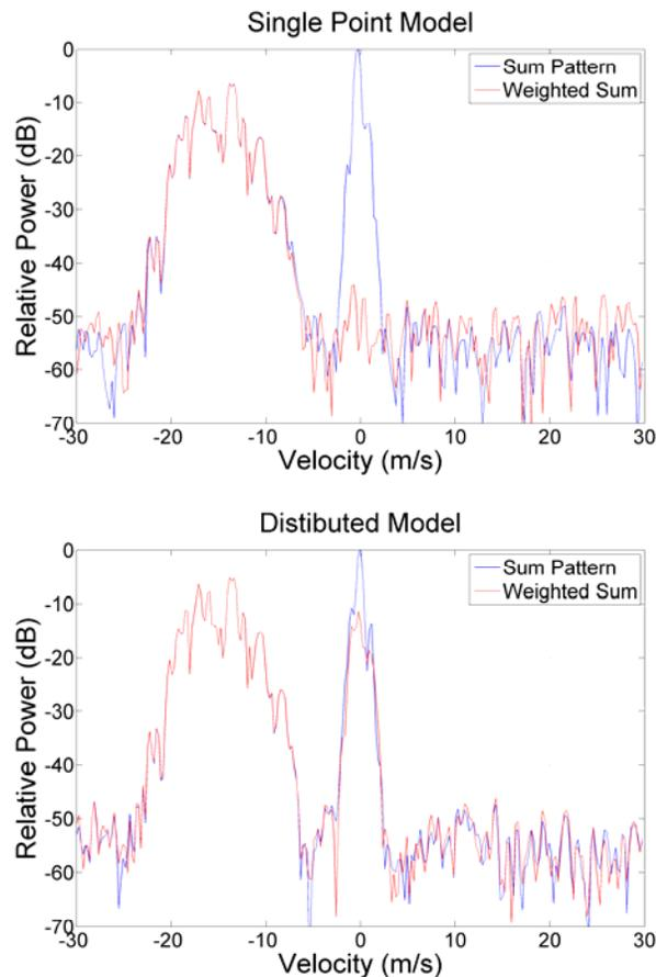
Figure 5. Spectra showing the performance of spatial filtering for both a single point and distributed clutter model.
