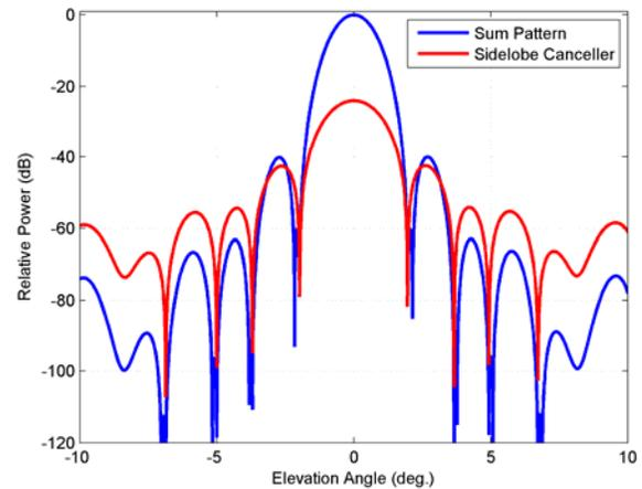
Figure 3. Theoretical antenna patterns calculated based on the location of the antenna elements and sidelobe canceller receive antennas.
