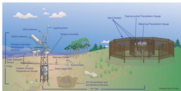
Figure 1: Schematic description of a US Climate reference Network station. Each station has the same design.
