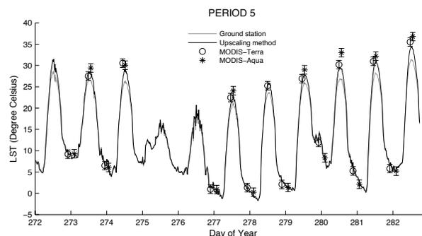
Figure 4: LST measured by a SURFRAD station (gray line) and by MODIS satellites (circles and stars), and assessed using the upscaling methodology (black line) over Bondville, IL. Error bars represent the possible errors associated with MODIS data – from MODIS quality flags.
