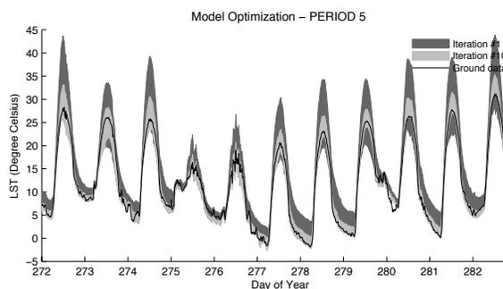
Figure 3: Look-up table of model simulations (LST values) generated by the calibration methodology. Every iteration of the MCIP algorithm represents an ensemble of 6,000 simulations. Ten iterations are used to minimize the bias and RMSE between observed (black line) and simulated LST. Results are for period 5.
