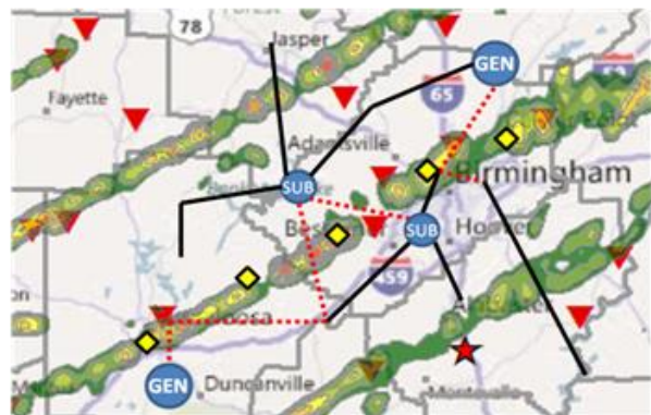
Figure 7. Conceptual overlay of weather and electrical power system showing tornado track detections (shading), tornado reports (triangles), power outages (diamonds), generating facilities (G), substations (sub), and main transmission lines (black and red dotted).
