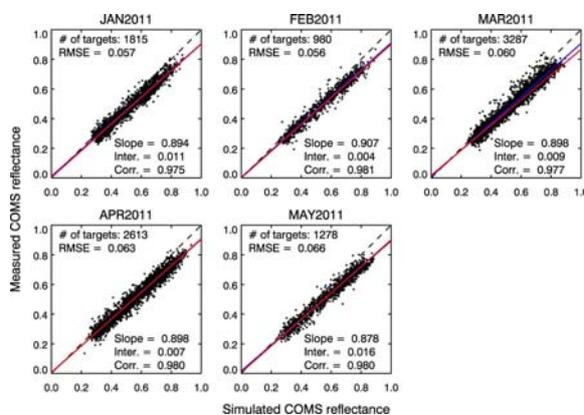
Fig. 2. Comparison between simulated COMS reflectances and measured COMS Level 1B reflectances. Regression lines from Methods 1 and 2 are given with red and blue lines, respectively.
