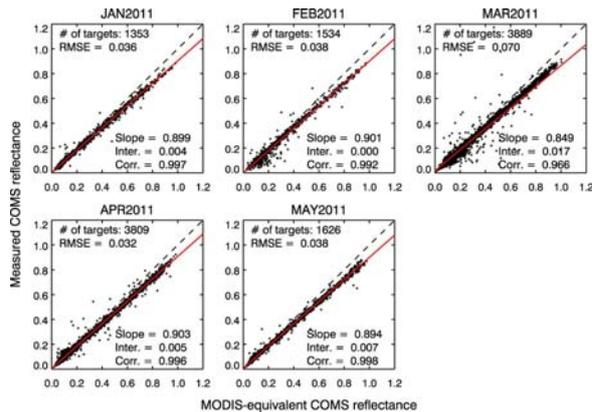
Fig. 1. Comparison between MODIS-equivalent COMS reflectances and measured COMS Level 1B reflectances.
