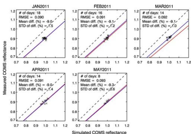
Figure 3. Comparison of Method 3 (crosses) against Method 1 (red line) and Method 2 (blue line). For Method 3, the daily average is calculated when the number of selected DCC targets is greater than 10.
