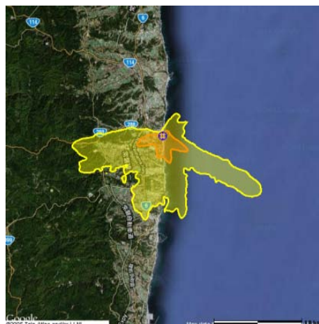
Figure 1. Example of the 14-day Total Effective Dose for a hypothetical release scenario. The color contours show the 1 (yellow) and 5 (orange) rem dose levels.
