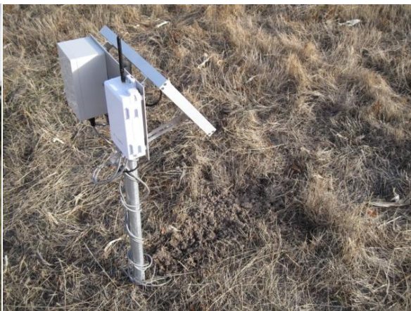
Soil sensors require equalization time
