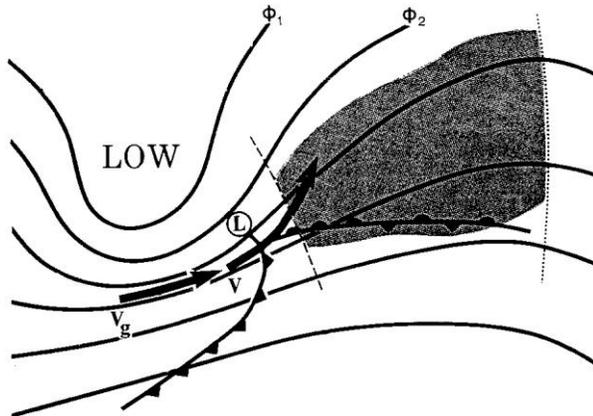
Fig. 10. Schematic of a typical mesoscale gravity wave formation pattern. V is the location of the 300-hPa jet streak, LOW is the center of the 300-hPa low, the solid lines are 300-hPa heights,  $V_g$  is the 300-hPa geostrophic wind maximum, the shaded region is the area of gravity wave formation. Surface features are also shown. From Koch and O'Handley (1997).
