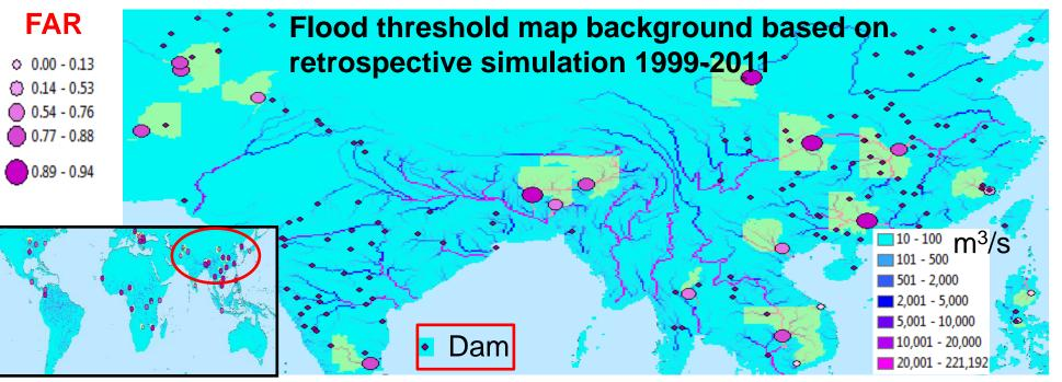
Fig. 6 Flood detection evaluation of the new GFMS over 49 well reported areas
