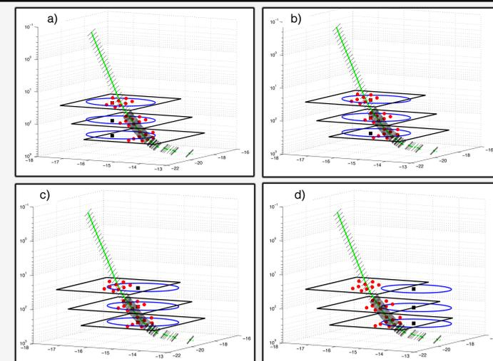
Figure 1. From left to right, AIRS a) 32.3 mb (AIRS Level 30), b) 103 mb (AIRS Level 44) and c) 300 mb (AIRS Level 63) temperatures differenced from the AIRS closest profile temperature (K) showing the closest profile (black square), circular averaged profile radius (magenta circle), ray averaged profiles (red dots), and the COSMIC RO raypath (black line).
