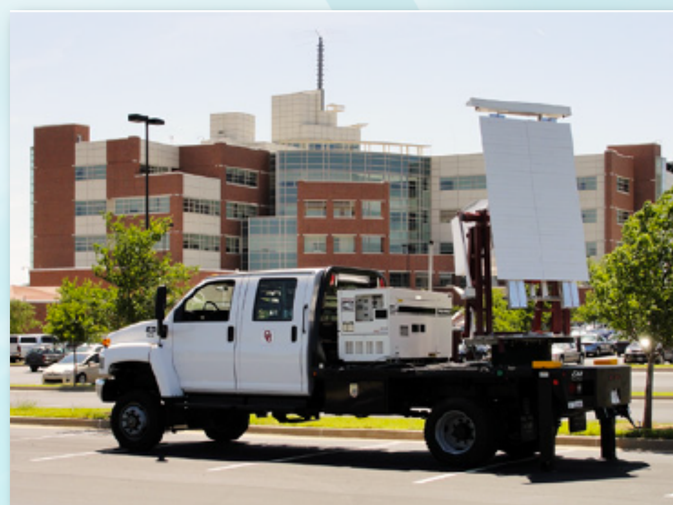
The Atmospheric Imaging Radar in front of the National Weather Center in Norman, OK. The system uses a fan-shaped transmit beam, and forms pencil beams on receive using digital beamforming.
