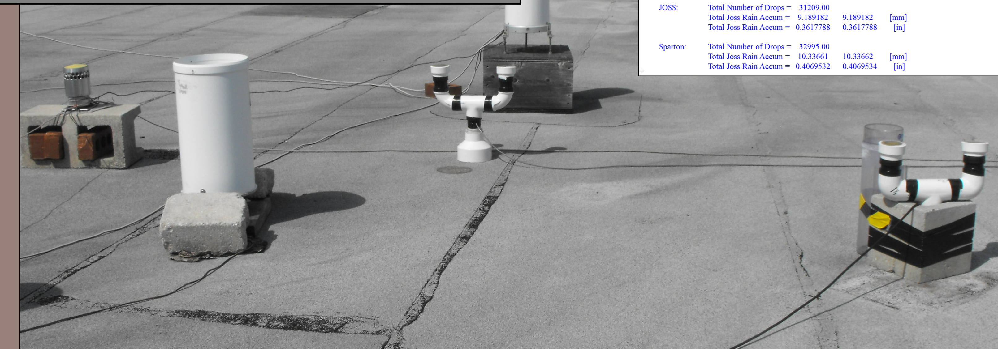
UCF disdrometer and radiometer test site (roof of Eng Bldg) – JWD on far left, experimental disdrometer (JTD) center and right.
