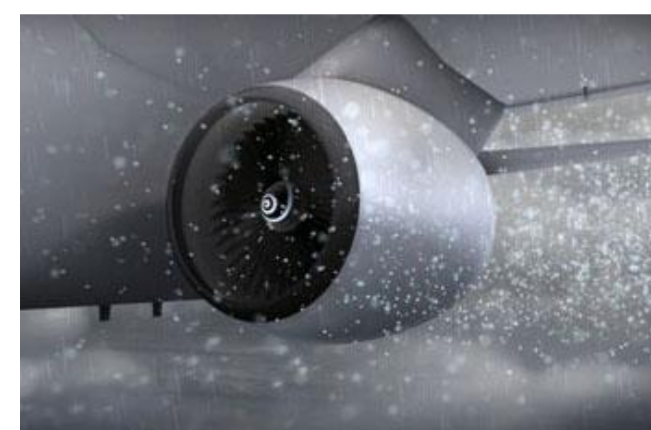
Jet engines are hypothesized to be susceptible to high concentrations of small ice crystals http://nasa-spacestation-info.blogspot.com/2011/08/airplane-plus-heat-plus-ice-equals.html
