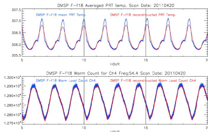
Fig. 1 F-18 PRT temperature (top) and warm count (bottom) for channel 4 on Apr. 20, 2011. Blue curve show the original data, and the red curves show the reconstructed data when signals with the frequency larger than the 2nd harmonics are filtered.
