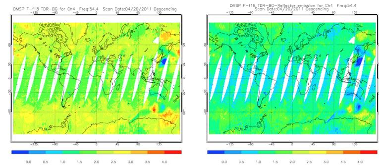
Fig. 5 Bias of observation from simulation (left) and bias of observation from simulation after removal of reflector emission (right) for channel 4 descending orbits on Apr. 20, 2011.
