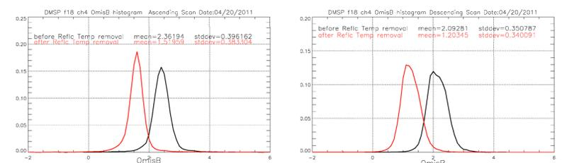
Fig. 6 Bias histogram for fig. 4 (left) and fig. 5 (right). The blue curve shows the histogram of bias before reflector emission removal and the red curve shows the histogram of bias after reflector emission removal.
