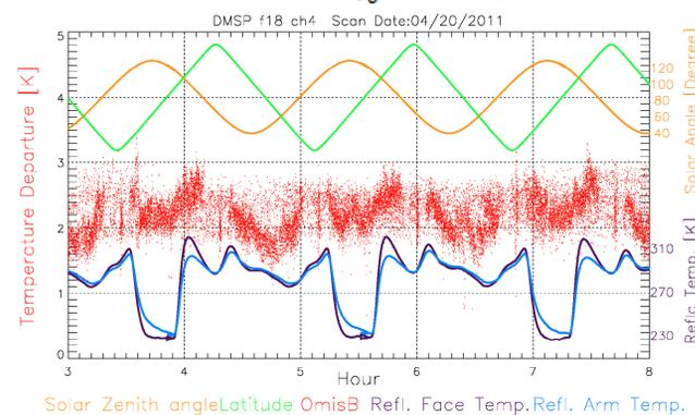
Fig. 3 Time series of latitude, solar zenith angle, OmisiB reflector face temperature, and reflector arm temperature
