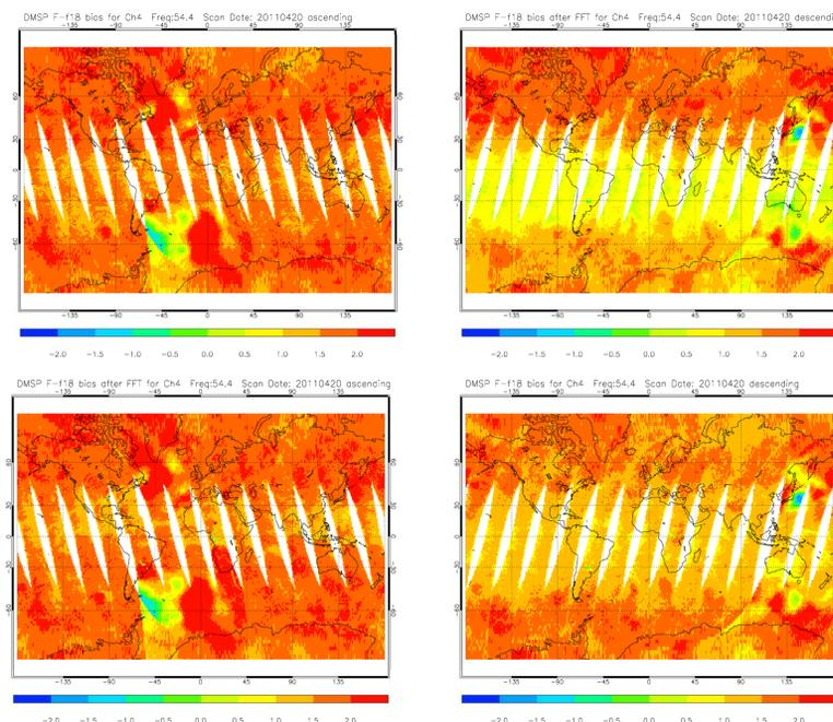
Fig. 2 Bias of observation from CRTM simulation for channel 4 on Apr. 20, 2011. Top: with original warm count and PRT temperature. Bottom: with reconstructed warm count and PRT temperature. Left: ascending orbits. Right: descending orbits
