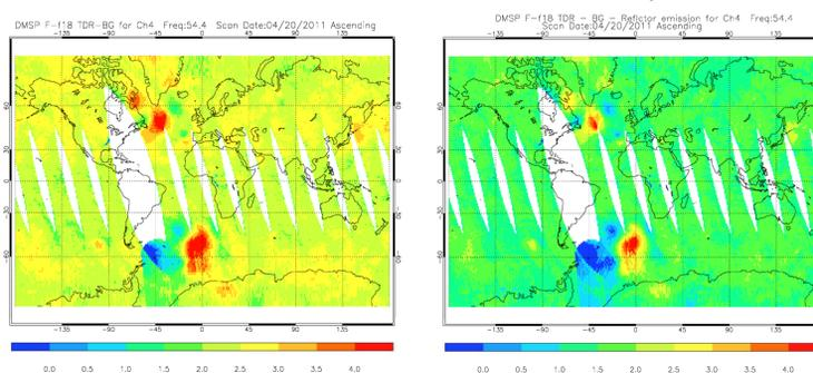
Fig. 4 Bias of observation from simulation (left) and bias of observation from simulation after removal of reflector emission (right) for channel 4 ascending orbits on Apr. 20, 2011.
