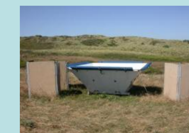
915MHz wind profiler and Radio Acoustic Sounding System (RASS)
