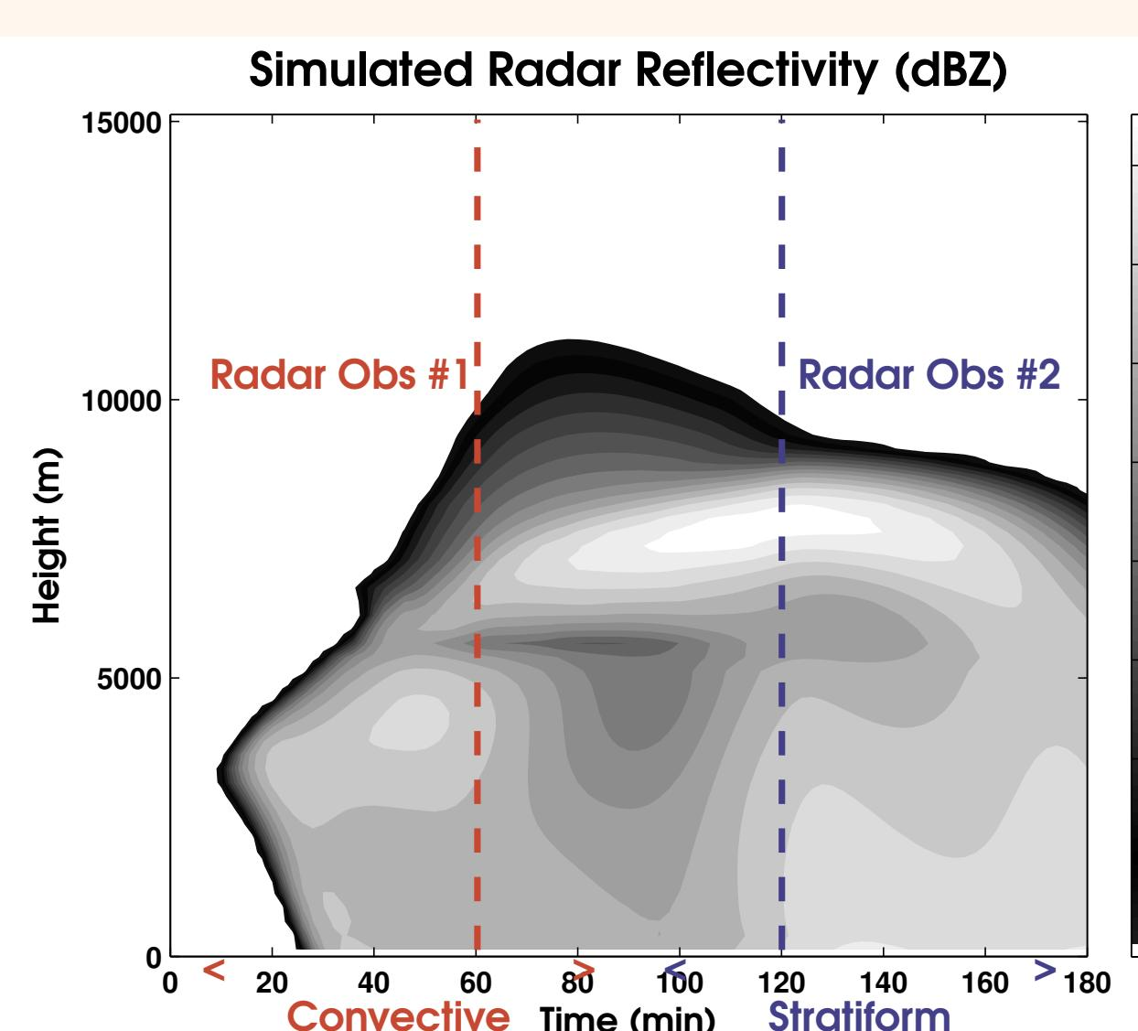
A 1-D idealized atmospheric column model with one moment bulk microphysics [4] is used to simulate microphysical processes present within a squall-line without dynamical or thermodynamical feedback. Simulated radar observations at 60 and 120 mins are produced by the Quickbeam [2] radar forward operator (shown for the "truth" run above). The observation times correspond to the convective and stratiform phases of the simulation.
