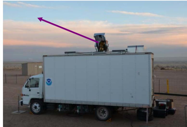
Fig. 1 Truck-based, scanning TOPAZ lidar at the 2012 Uintah Basin study.
