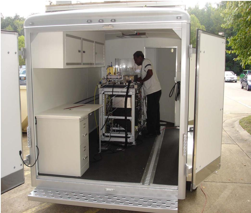
**NASA Langley** is developing an ozone lidar in a trailer that can be easily deployed at locations throughout the U.S. The lidar will produce tunable on and off ozone DIAL laser wavelengths between 280 and 300 nm at 500 Hz each. There is also a 527 nm aerosol channel. The system has an in situ ozone measurement capability which will allow ozone to be profiled from the ground to the lower troposphere.
