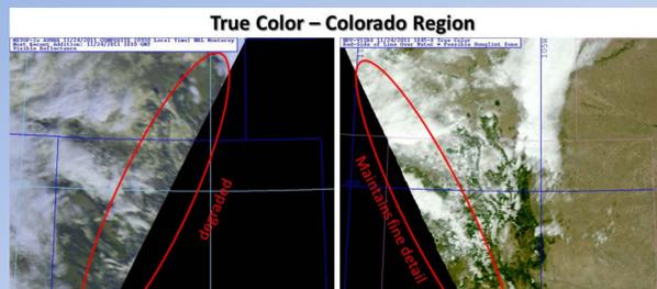
VIIRS borrows from DMSP OLS cross-track scanning technology that maintains the fine detail from nadir to edge of scan. In contrast, MODIS and AVHRR imagery become increasingly degraded away from nadir.
