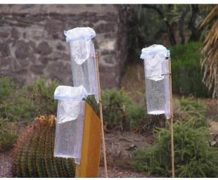
Wet deposition with rain gauge
