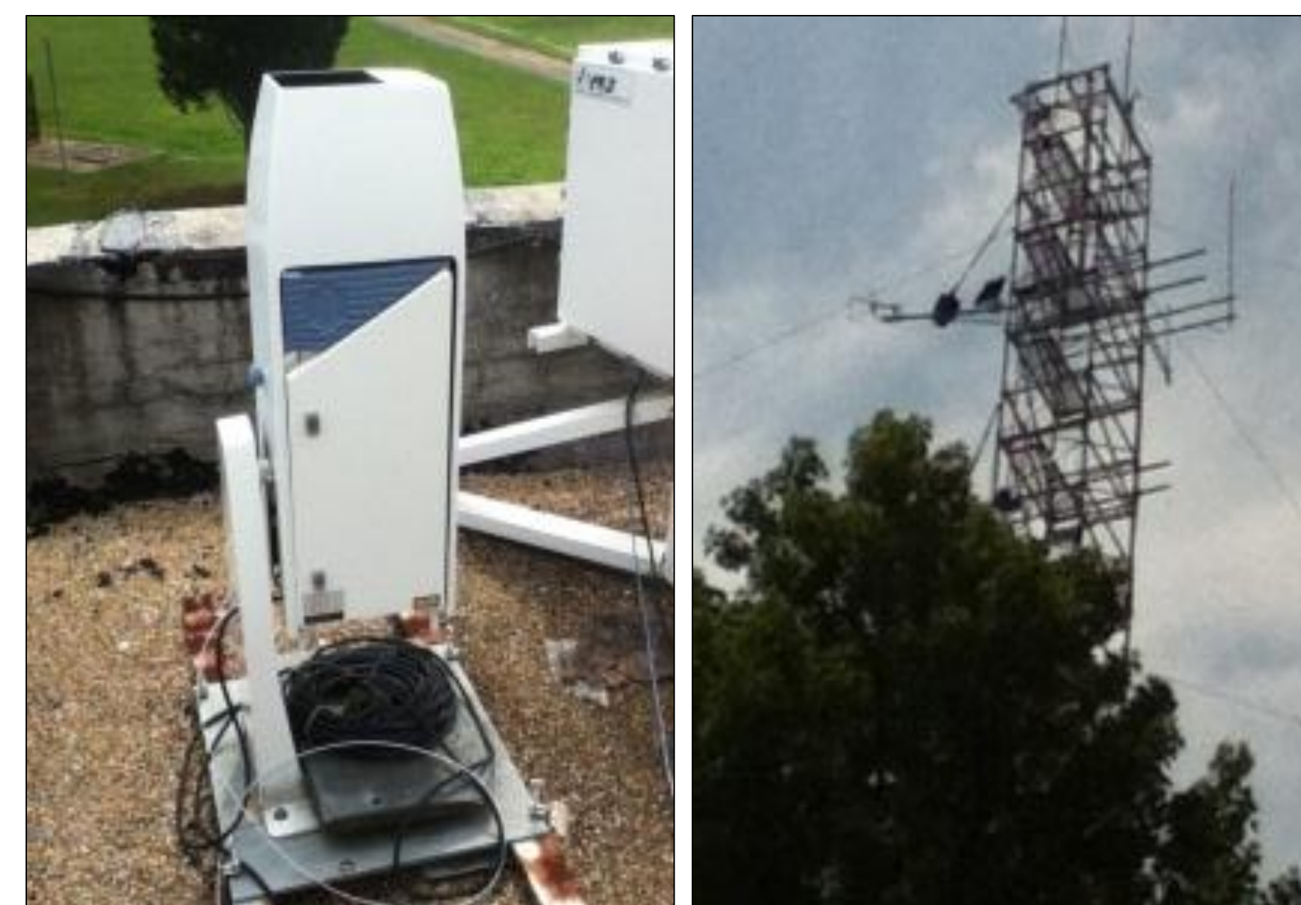
Figure 2: The ceilometer (left) and 31-meter flux tower (right) used in this study. Both are located on site at the BCCSO.
