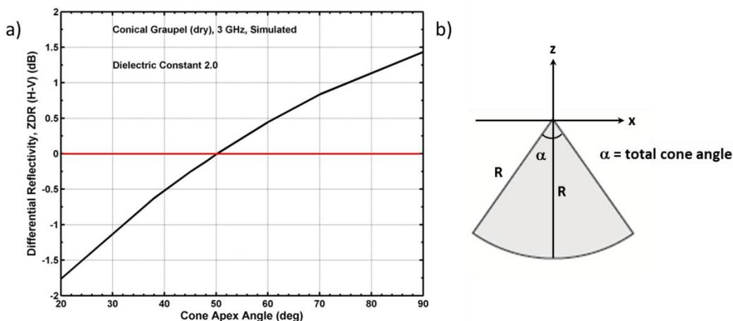
Figure 11. a)  $Z_{dr}$  as a function of the apex angle for the curved base model. Calculation details are the same as figure 10. b) Schematic shape of the conical graupel with curved base.
