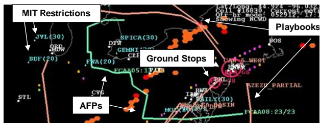
Figure 2. A sample of TMIs that can explicitly modeled or enforced in DART.
