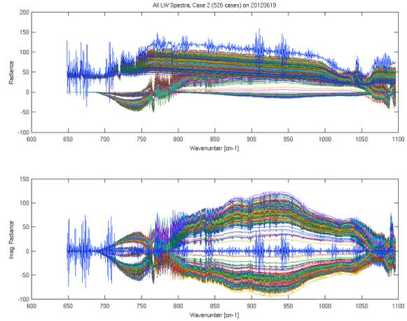
Figure 7. Case 2 flagged LW CrIS spectra on 19 Jun 2012. Real and imaginary radiances are provided (top and bottom panels, respectively).
