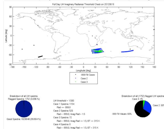
Figure 3. CrIS LW QA image for analysis on 19 June 2012. Image shows spectra that have been flagged using the imaginary radiance threshold check.
