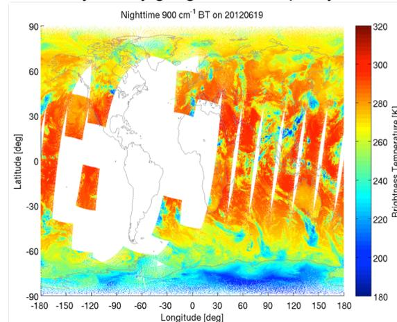
Figure 4. Nighttime 900 cm<sup>-1</sup> T<sub>b</sub> on 19 June 2012. Gaps in the data are due to missing data from repair-granules that have not been packaged into the final CrIS SDRs.
