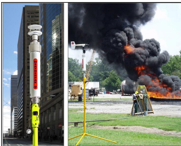
Figure 5. Two examples of HAZMAT meteorological sensor suites: WEATHERPAK MTR (left) and WEATHERPAK TRx (right). (Hemmingway, 2012)
