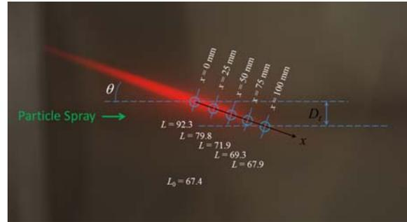
Figure 9. Side scatter measurements through lunar dust simulant.
