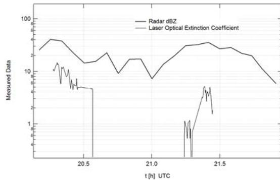
Figure 16. October 2, 2012 rainfall event at Pine Island, FL. Normal width line is the optical extinction coefficient measured by the laser system; bold line is the average of the nearest four bins of radar reflectivity from Melbourne NEXRAD (lowest elevation scan) over the laser site shown in Figure 8.
