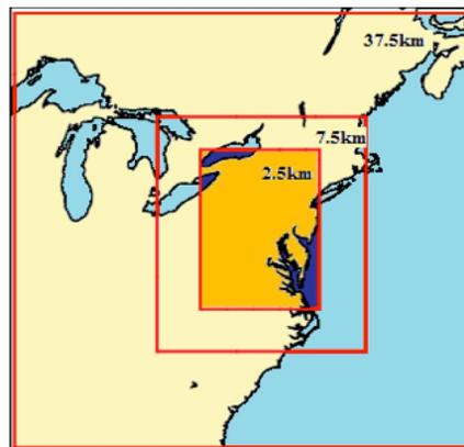
**FIG 1. Model experimental domain (shaded) over the Chesapeake Bay watershed, shown along with the three-grid nesting configuration that is used. The outermost grid resolution is 37.5 km, the middle grid is 7.5 km and the innermost grid resolution is 2.5 km.**
