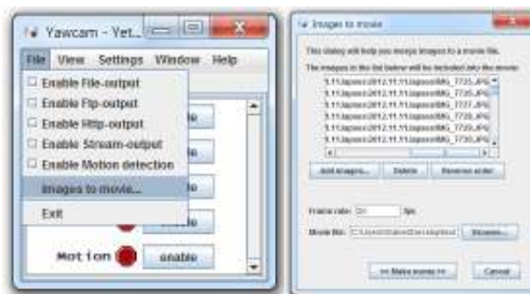
Figure 3. Yawcam interface demonstrating the "Images to movie" option that allows a user to quickly select a sequence of images, add a frame rate (frames per second, of fps), and generate a .mov format ready for playback in players that support that format (e.g., QuickTime, Windows Movie Player). This feature is useful for creating movies of specific features or set periods of the day. Alternatively, this software tool can be used to create lapses of any setting that includes a series of images shot using a DSLR, an intervalometer, and a tripod. The first author uses this method for time-lapse movie creation of cloudscapes acquired during storm chases.
