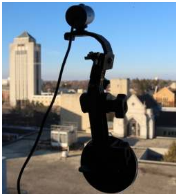
Figure 5. "North" webcam on window suction cup mount providing high-resolution images with 10 second updates.
