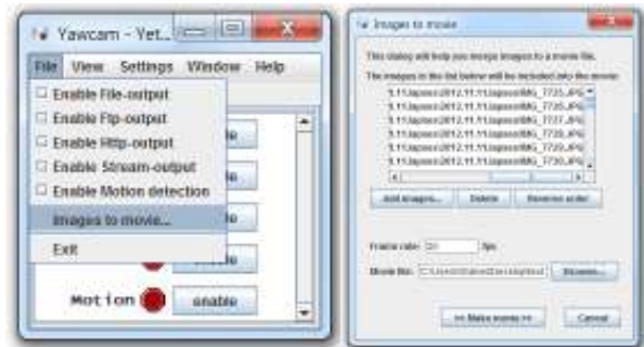
Figure 3. Yawcam interface demonstrating the "Images to movie" option that allows an user to quickly select a sequence of images, add a frame rate (frames per second, of fps), and generate a .mov format ready for playback in players that support that format (e.g., QuickTime, Windows Movie Player). This feature is useful for creating movies of specific features or set periods of the day. Alternatively, this software tool can be used to create lapses of any setting that includes a series of images shot using a DSLR, an intervalometer, and a tripod. The first author uses this method for time-lapse movie creation of cloudscapes acquired during storm chases.
