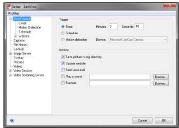
Figure 4. Tin Cam "Setup" interface. Menu on left reveals the numerous configuration options; in this example, "auto capture" is set to take an image every 10 seconds, save it to a log directory, and update website (which also pushes FTP).
