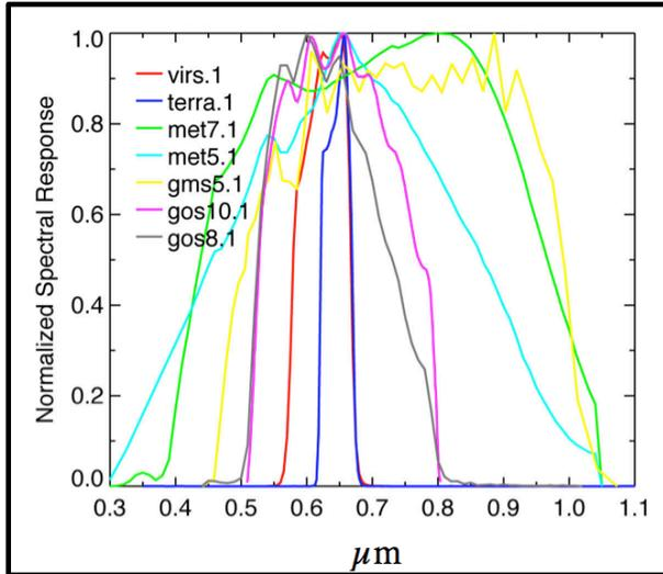
Figure 1. The visible spectral response functions of five geostationary satellites along with the MODIS  $0.65\mu\text{m}$  channel onboard Terra and VIRS onboard TRMM. Note that Terra has a much narrower spectral response function.
