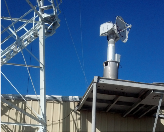
FIG. 3. A photograph of the Ranger-X1 in Enterprise, AL. The location of the radar provided reasonable coverage, though some blockage was incurred due to a nearby tower.
