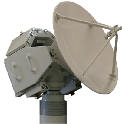
FIG. 2. A photograph of the Ranger-X1 prototype radar. The 1-m dish and polarimetric feed are shown, along with one of the two transceiver enclosures (other is hidden on opposing side). The pedestal structure is sealed against the elements, which is ideal for continuous outdoor operation.
