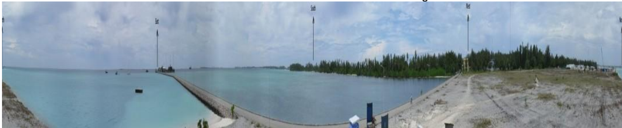
Fig. 2: Panoramic image taken from the S-Pol pedestal, 3 m below the center of the dish; north is at each edge, and the vertical scale has been exaggerated by a factor of four to better show variations in the blockage.
