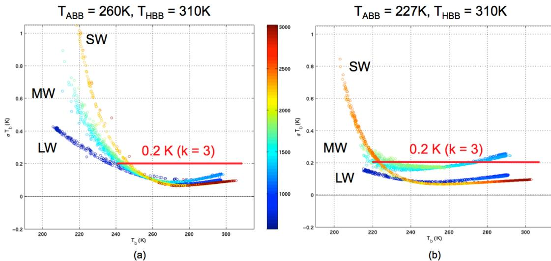
Figure 4: S-HIS calibration uncertainty estimates ( $k = 3$ ) for flight conditions encountered on (a) 21 November 2002 on the ER-2 and (b) 16 November 2002 on the Proteus [11 – 12].
