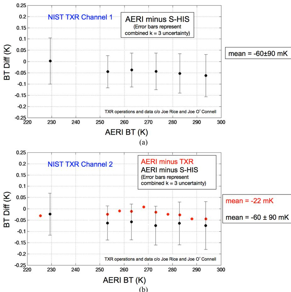
Figure 5: NIST TXR comparison results; (a) NIST TXR Channel 1 (5 μm) (b) NIST TXR Channel 2 (10 μm) [6 – 10].
