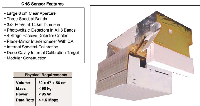
Figure 1: The Cross-track Infrared Sounder (CrIS) [3].
