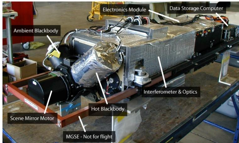
Figure 2: The Scanning High-resolution Interferometer Scanner (S-HIS); Proteus integration, Scaled Composites, July 2004.
