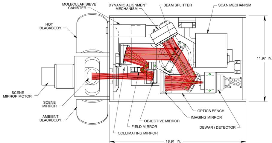
Figure 3: Diagram of the S-HIS interferometer module and flight calibrator assembly viewed from the nadir perspective. The Zemax prescribed IR beams are shown, and have been omitted from the figure between the beamsplitter and the Michelson mirror.
