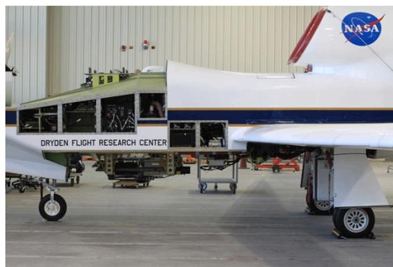
Figure 6: The S-HIS mounted in Zone 25 of the NASA Global Hawk for the NASA Hurricane and Severe Storm Sentinel (HS3) mission.
